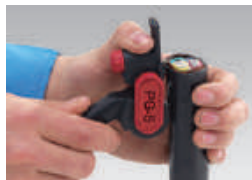
设定工具纵向切割 Put the tool vertically
