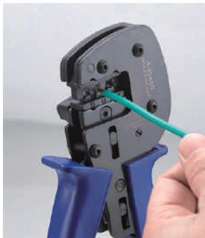
接着把已剥皮绝缘导线放进端子 Then put the stripped insulated conductor into the terminal
